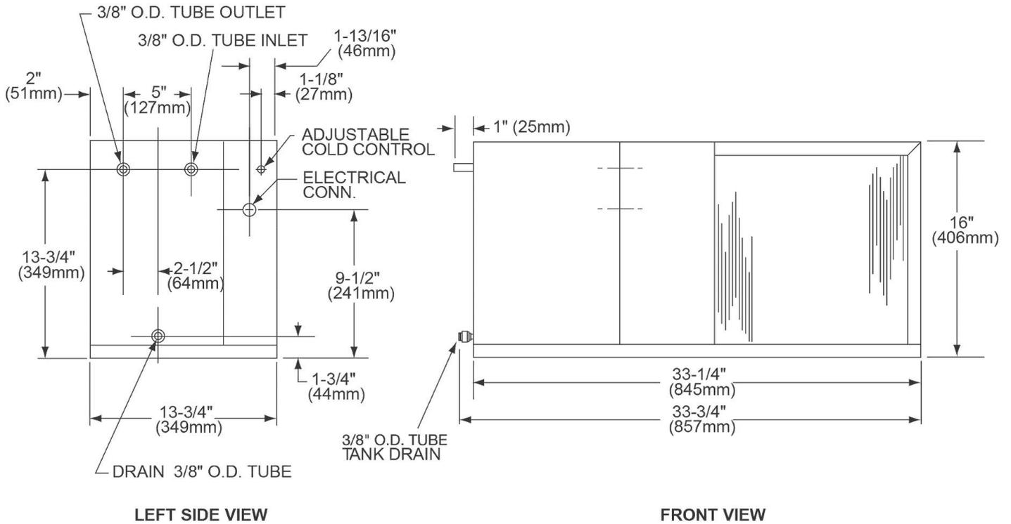
**NOTE:** This unit is intended for remote installation only. It is important to insure proper ventilation. Allow a minimum clearance of 6"(152mm) in front and 6"(152mm) in the rear of unit.
